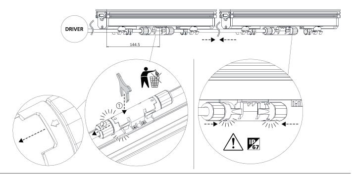
Periodically check for water accumulation inside the housing. The Presence of water is a symptom of non-compliant installation. Any faults arising under these conditions shall not be covered by the waranty. It is essential to periodically clean the glass. There should be no accumulation of dirt, leaves, limescale, etc. This would inhibit both heat dissipation and light emission.
